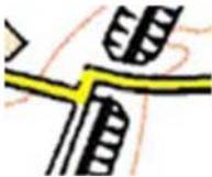
**A yellow road going Over a Railway (RO). Note the white space between the yellow road and the bridge symbol integrated with the embankment.**
